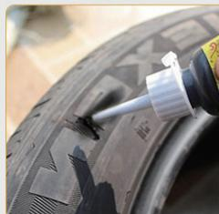
Clean up particles and dust and apply tire glue
