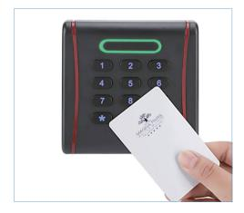
Hitag2 chip card, one of LF Proximity Card, operates on 125 kHz. Compared to the other 125 kHz RFID cards, the Hitag2 chip card is a little expensive, but it has better safety performance and RF performance. It has a storage capacity of 256 bits and the data may be transmitted enciphered.
