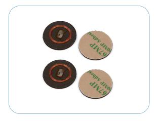
Anti-metal Ntag216 NFC Coin tag belongs to the NFC anti-metal tag family, which works well on the metal surface. This tag stands out from NFC anti-metal tags because of its chip-Ntag216 with a larger storage capacity: 924 bytes of total memory and 888 bytes of user memory. And it has another feature that is similar in shape and size to coins.
